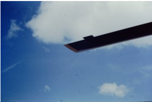
Main rotor blade with small arms holes
