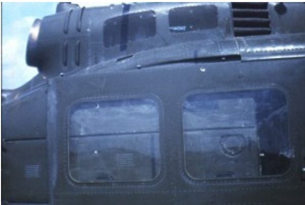
Pilot's side of the aircraft with numerous bullet holes
