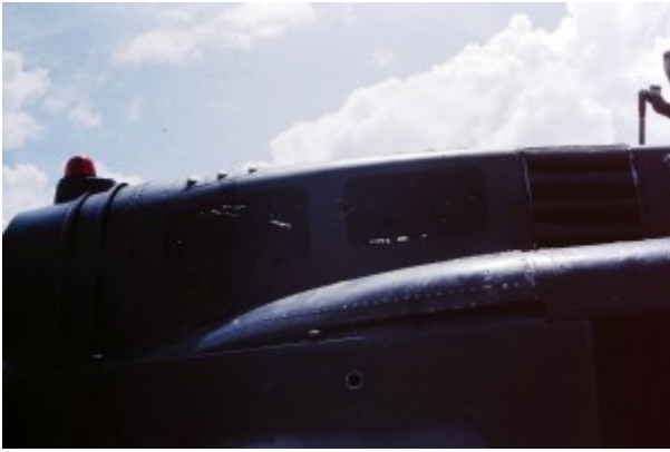
AC side of aircraft engine deck with numerous bullet holes
