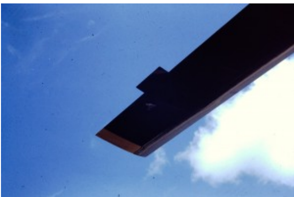
Main rotor blade with 12.7mm (50 cal) hole
